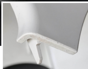
BEFORE CLEANING: Part contamination by mold residues
