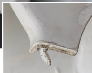
DURING CLEANING: Heavily contaminated part pulled from mold after application of Lusin® MC1718/1719
