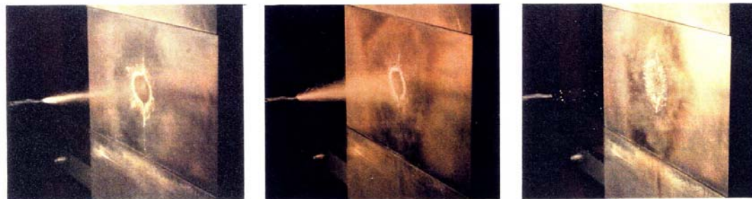
Figure 12: Photographic comparison of three die lubricants during spraying onto die steel. The initial temperature of the die steel was 340°C. The time between photographs is 0.6 seconds.
