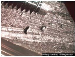
Fig 2: Shrinkage porosity
