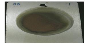
After exposure, there is only minor corrosion in the land areas of the panel, but most noticeably, the area where the disc has been molded has turned a rusty red color. This is a clear indication that even an anti-moisture barrier cannot totally isolate the metal from atmospheric oxygen and moisture
