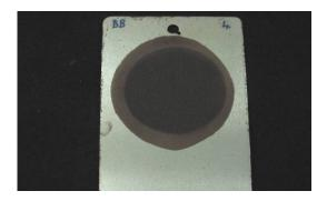
After exposure, the land areas of the panel were quite heavily corroded. The disc that had been in contact with molded rubber was red rusty, once again indicting the profound effect of the halogenated compound at the mold surface.
