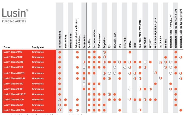
In case of material change from A to B purge with Lusin® purging compound suitable for A
