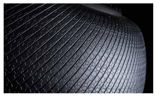
unfilled tire paints create a reservoir of slip-and-release functionality on the curing bladder surface, which then permits the release of several untreated tires between applications.
